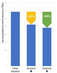
Retro-fitting all uninsulated components of the pipe systems could reduce energy losses by more than 20%<sup>(3)</sup>
